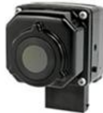
(f) Thermal Camera FLIR PathFindIR
