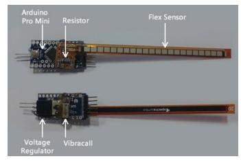
Fig. 6. Prototype of the Postural Electronic Corrector
